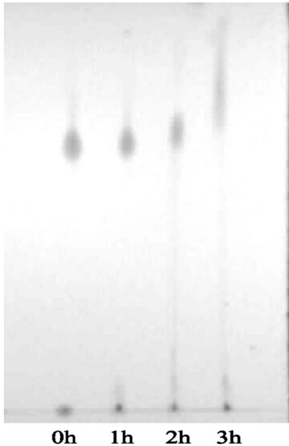
Fig. 8 Thin-layer chromatogram of the hydrolysis products of phytate with the crude phytase produced by the marine yeast strain used in this study. Lane 1 : phytate+the crude phytase within 0 h); lane 2 : the hydrolysis products for 1 h; lane 3 : the hydrolysis products for 2 h; lane 4 : the hydrolysis products for 3 h. The end products of phytate hydrolysis were analyzed by using a TLC plate (Silica gel 60, MERCK, Germany) with the solvent system 160 ml of chloroform, 60 ml of acetone, 52 ml of methanol, 48 ml of glacial acetic acid, and 28 ml of water. The spots were located by exposing the plates to iodine vapor
